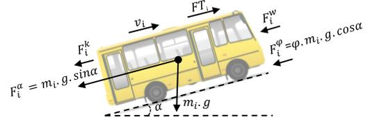
Fig. 2. Forces analysis for the vehicle of type  $i$ .
