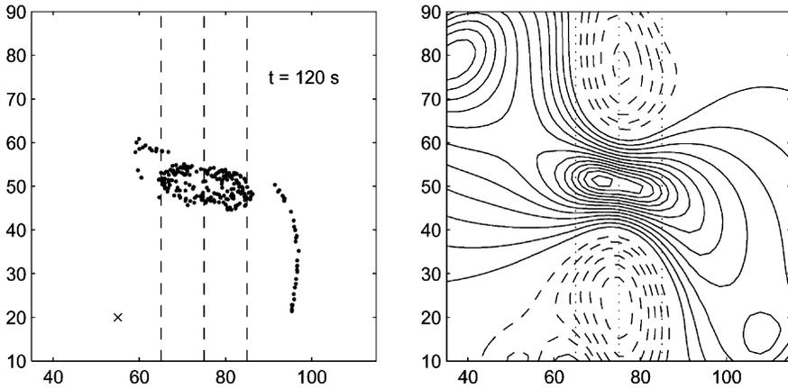
Fig. 10. Elliptical deformation of a vortex on top of the ridge at  $t = 120$  s. The flow parameters are:  $H_0 = 18$  cm,  $h_r = 3$  cm and  $W = 10$  cm,  $\Gamma = 100 \text{ cm}^2 \text{ s}^{-1}$ ,  $R = 2.5$  cm,  $x_0 = 55$  cm. Left panel shows 500 passive tracers initially placed in a circle of radius 7 cm and centred at the vortex core. Right panel presents stream function contours at  $t = 120$  s.
