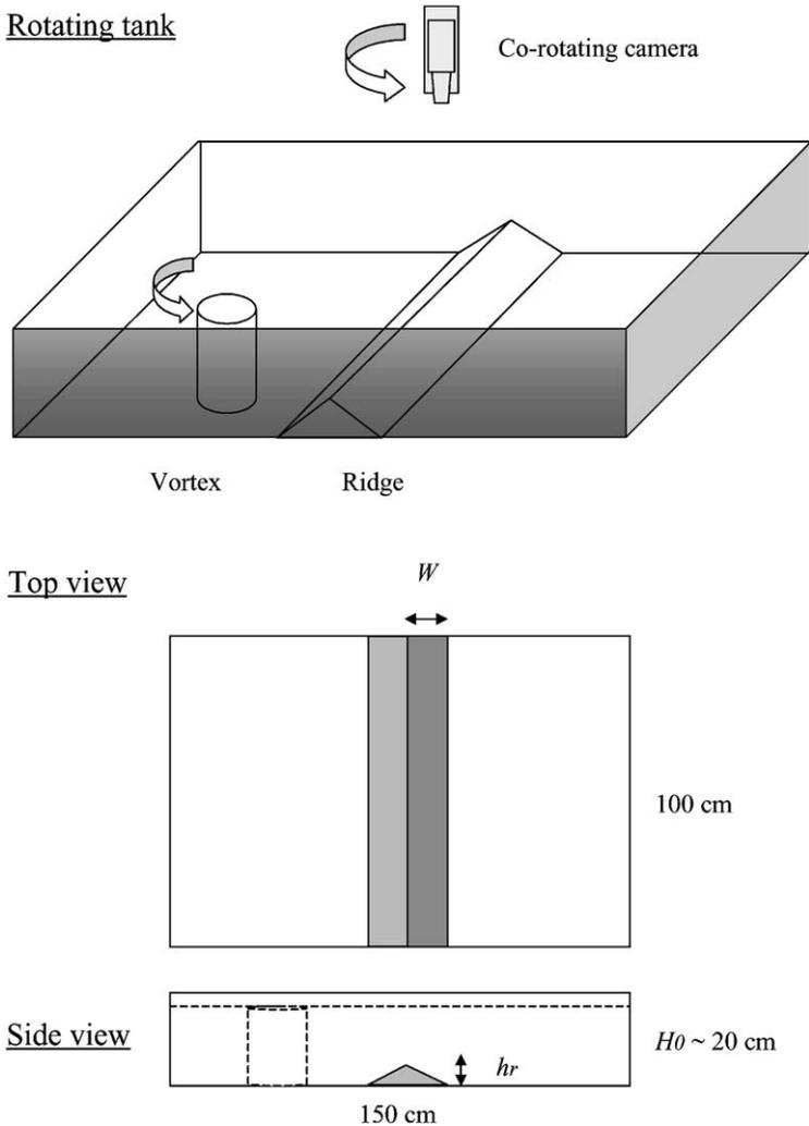
Fig. 1. Schematic view of the experimental arrangement. Cyclonic vortices are produced at the left-hand side (seen from above) of the triangle-shaped ridge.
