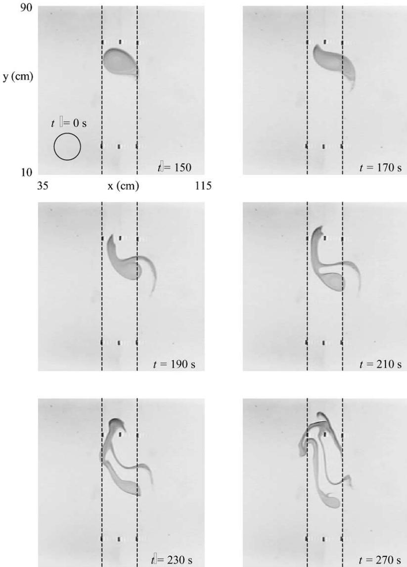
Fig. 4. Top view photographs showing the evolution of a vortex during a strong interaction on a  $f$ -plane. The parameters are  $h_r = 3$  cm and  $W = 10$  cm,  $H_0 = 23$  cm and  $x_0 = 50$  cm. The vortex trajectory, crossing the ridge one time, is plotted in Fig. 3a.
