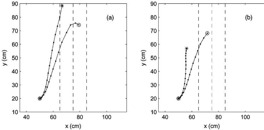
Fig. 7. Numerically calculated trajectories of a cyclonic vortex from  $t = 0$  to 140 s, every 10 s, when the depth fluid is  $H_0 = 12$  cm (\*) and 18 cm (○). (a) In the absence of bottom friction. (b) Including bottom friction. The vortex parameters are  $\Gamma = 80 \text{ cm}^2 \text{ s}^{-1}$  and  $R = 2.5$  cm. The ridge parameters are  $h_r = 3$  cm and  $W = 10$  cm.
