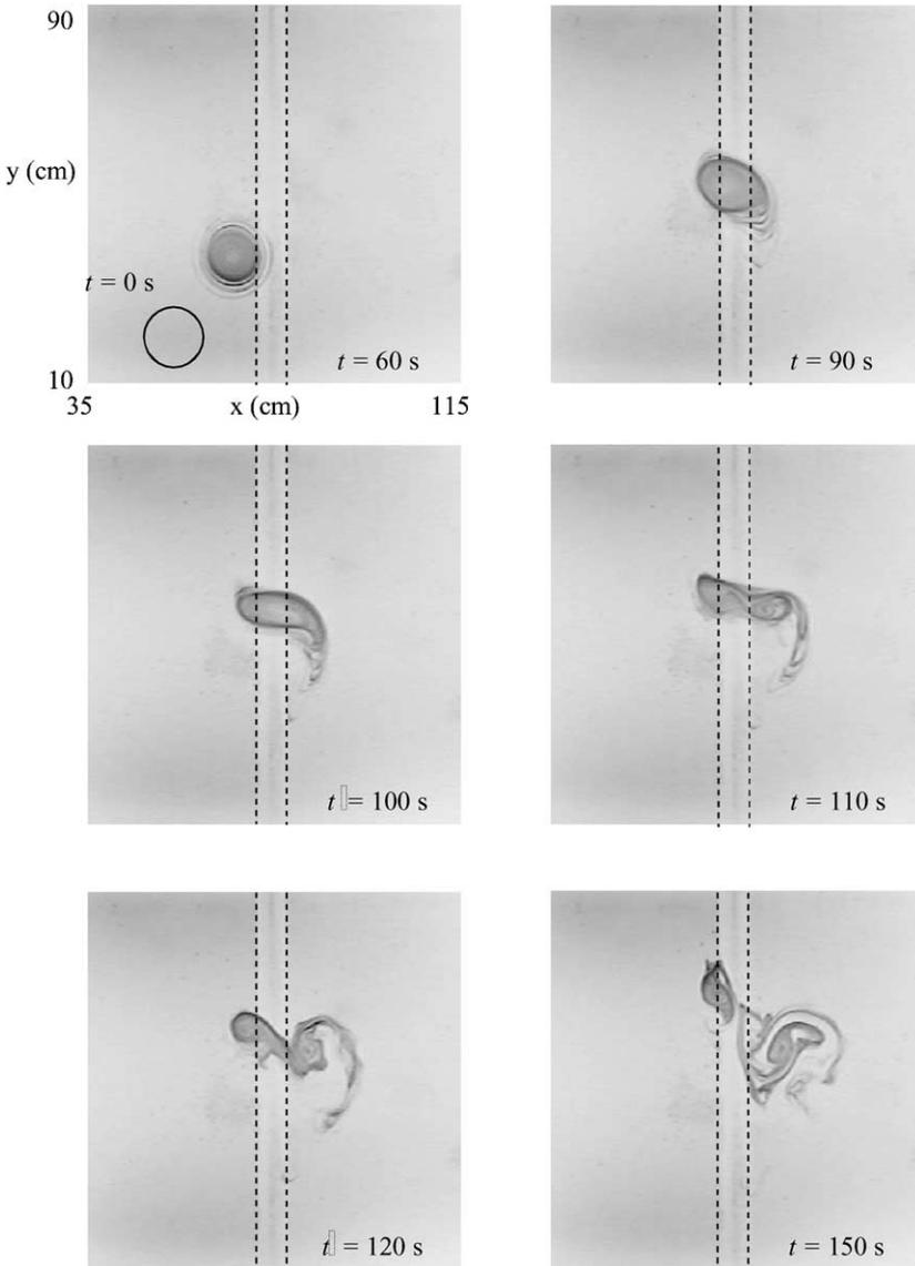
Fig. 6. Top view photographs showing the evolution of a vortex during a strong interaction over a narrow ridge. The vortex cleavage occurs at  $t = 110$  s. The parameters are  $h_r = 3$  cm and  $W = 5$  cm,  $H_0 = 21$  cm and  $x_0 = 60$  cm.
