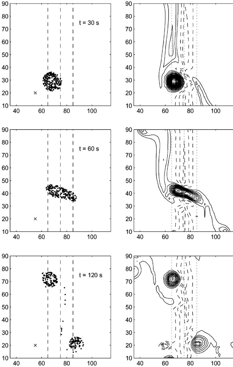
Fig. 11. Vortex cleavage during a strong vortex–ridge interaction. Left column shows the evolution of 500 tracers. Right column presents vorticity contours (with an interval of  $0.1 \text{ s}^{-1}$ ). The flow parameters are:  $H_0 = 18$ ,  $h_r = 3$  and  $W = 10 \text{ cm}$ ,  $\Gamma = 120 \text{ cm}^2 \text{ s}^{-1}$ ,  $R = 4.5 \text{ cm}$ ,  $x_0 = 55 \text{ cm}$ .
