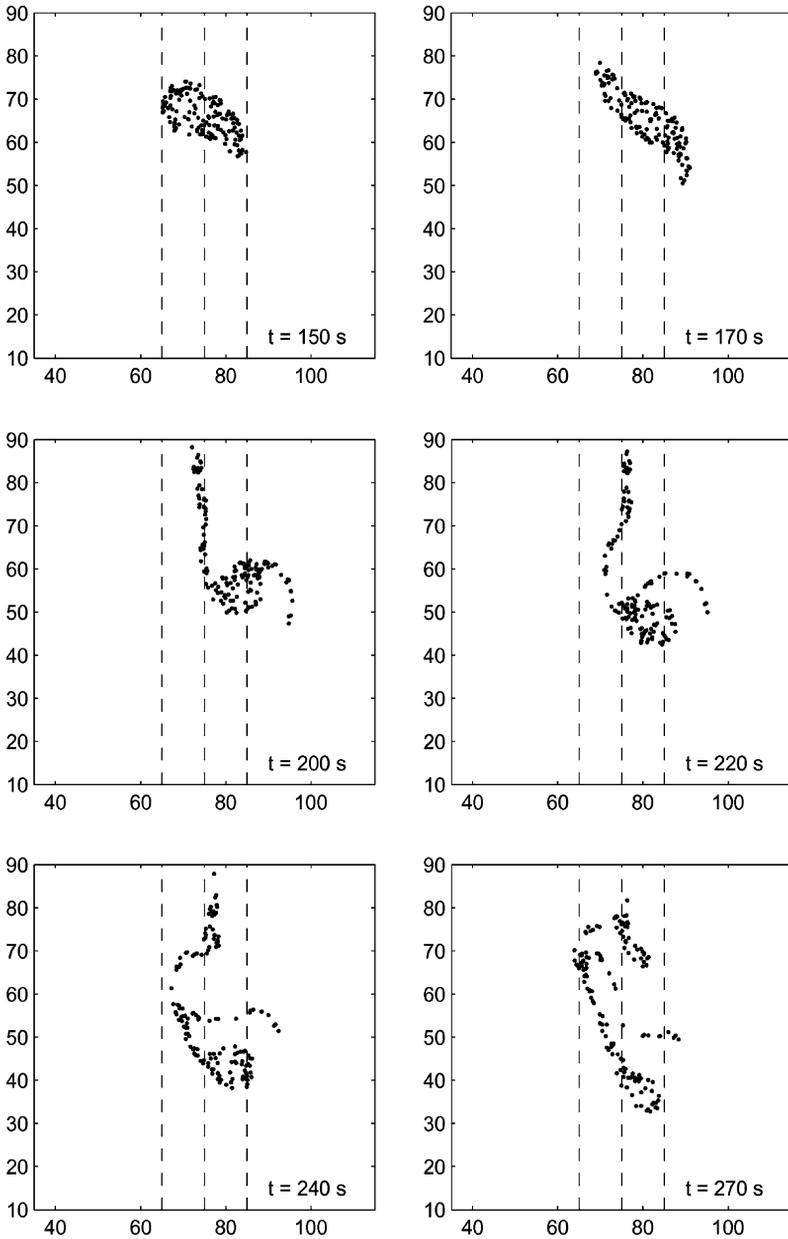
Fig. 9. Evolution of 500 tracers initially placed in a circle of radius 7 cm and centred at the vortex core, showing a strong interaction comparable with the experiment in Fig. 4. The flow parameters are:  $H_0 = 18$  cm,  $h_t = 3$  cm and  $W = 10$  cm,  $\Gamma = 80 \text{ cm}^2 \text{ s}^{-1}$ ,  $R = 2.5$  cm,  $x_0 = 50$  cm.
