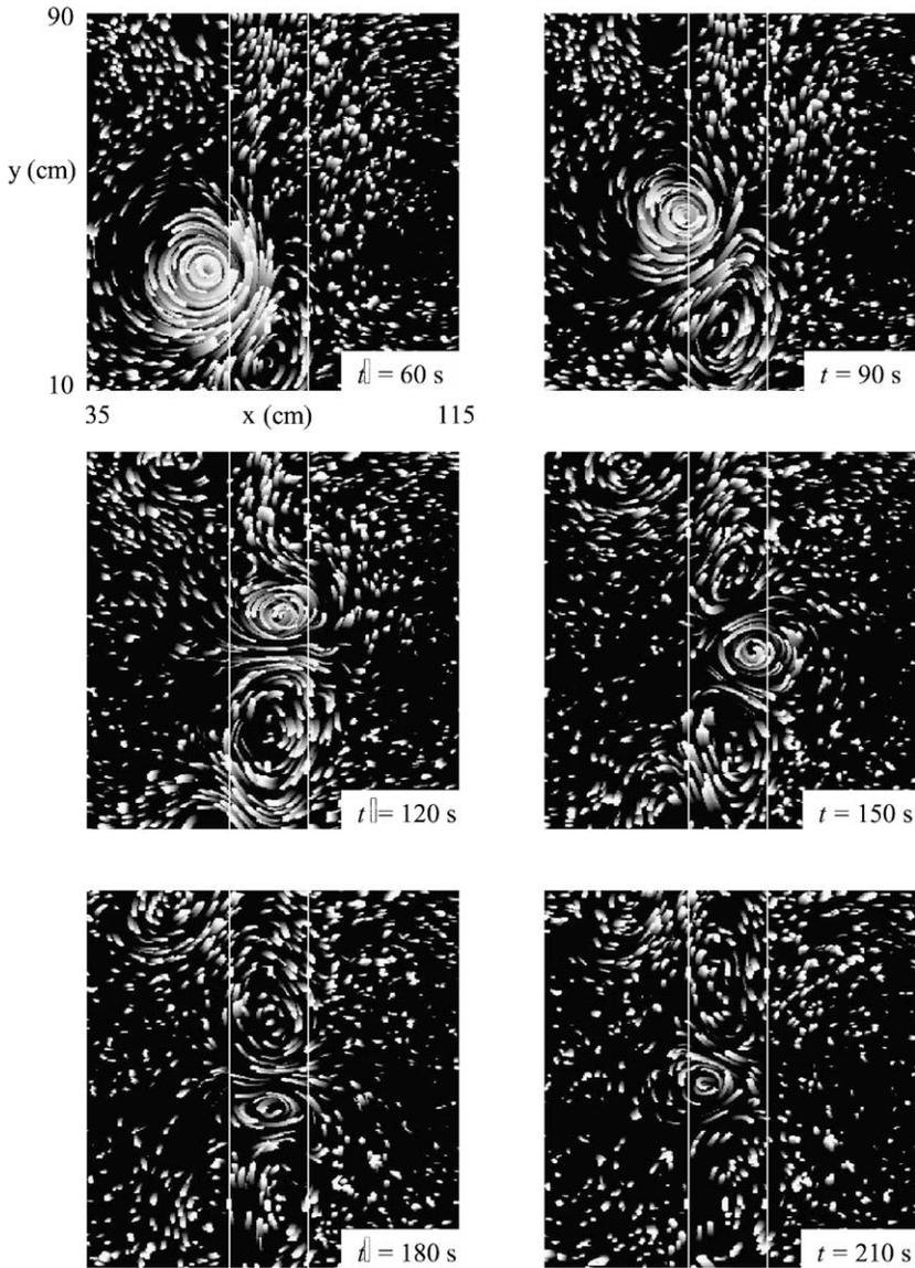
Fig. 5. Particle streak recordings of a cyclonic vortex during a strong interaction. White lines show the edges of the ridge. The elliptical deformation is produced after  $t = 120$  s. The flow parameters are  $h_r = 3$  cm,  $W = 10$  cm,  $H_0 = 21$  cm,  $x_0 = 55$  cm,  $\Gamma = 100$  cm<sup>2</sup> s<sup>-1</sup> and  $R = 2.5$  cm, approximately.
