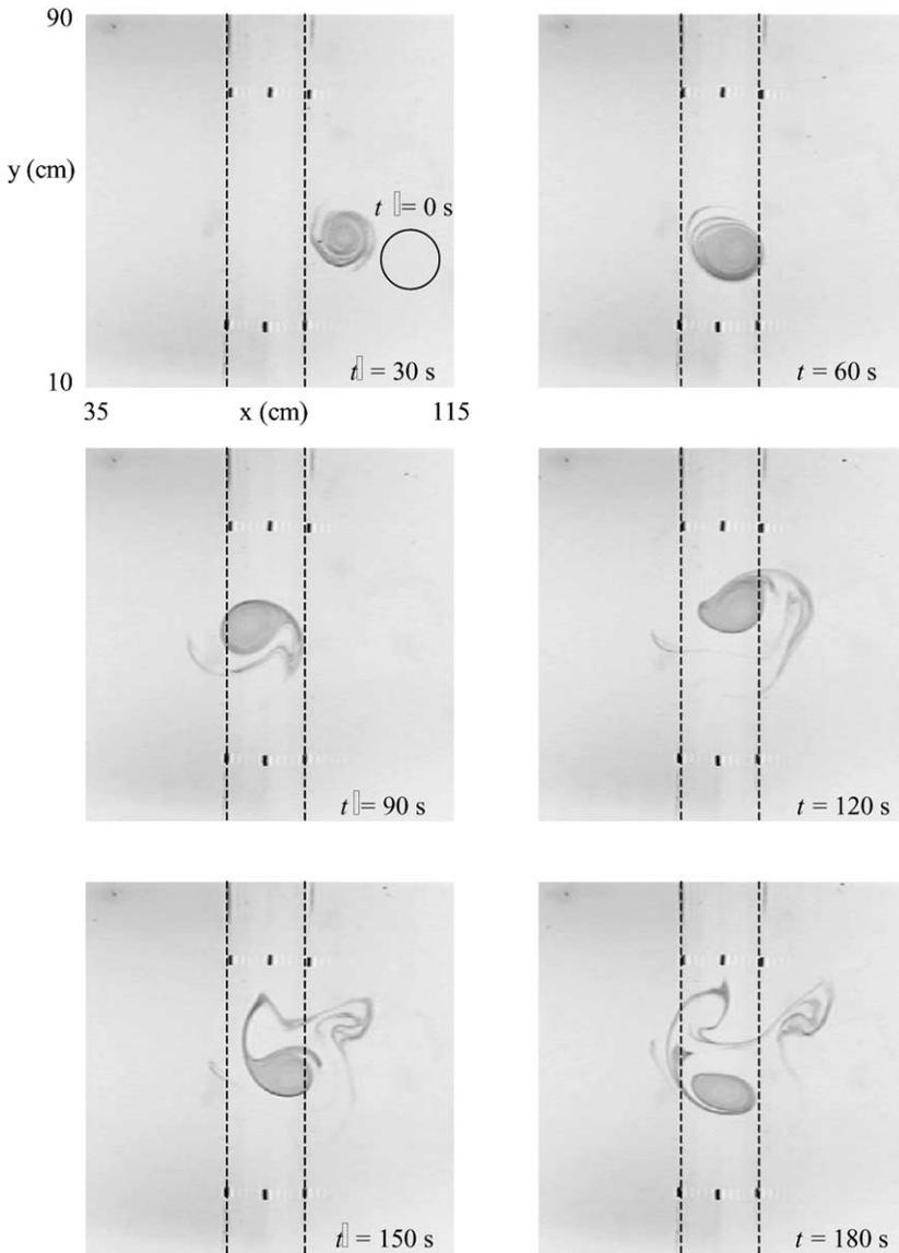
Fig. 12. Top view photographs showing the evolution of a vortex on a topographic  $\beta$ -plane. The initial position is at the eastern (right) part of the figure ( $x_0, y_0 = 105, 40$ ) cm. The ridge parameters are  $h_r = 3$  cm,  $W = 10$  cm.
